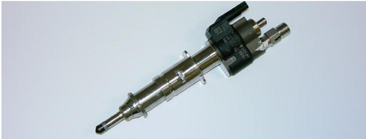
The piezo-injector is integrated together with the spark plug centrally between the inlet and exhaust valves in the cylinder head. This installation position prevents the cylinder walls or the piston crown from being wetted with injected fuel. A uniform formation of the homogeneous air/fuel mixture is obtained with the aid of the gas movement in the combustion chamber and a stable fuel spray cone.
