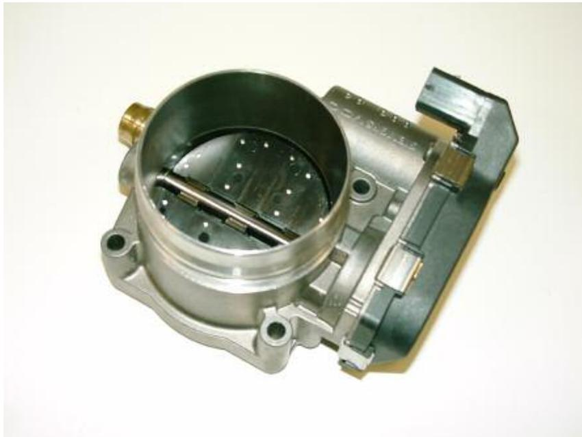
The magneto-resistive sensors are integrated into the housing cover. This sensor allows throttle position feedback to achieve an extremely high degree of accuracy.
