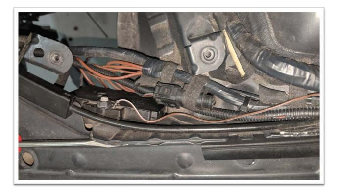
Run the harness all the way to the rubber gromet behind the DSC module. I poked a small hole through the rubber and ran the wires through. You will need to remove the driver's side under panel. I ran power from my deleted cigarette outlet but you could also run power from the fuse box. It needs to be from a 10-amp fused power source with 18-gauge wire. Pin in the signal wire to the CAS and tap the P Can lines from the LTM. I used heat shrinked butt connectors to tap the P can lines.
