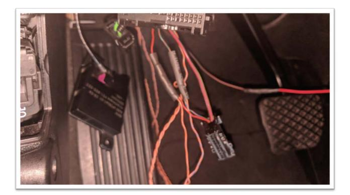
Neatly route the wires and reinstall the under panel. I zip tied the wires to the main wiring harness.
