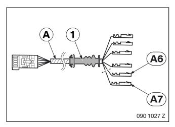
Carefully cut the rubber grommet (1) off retrofit cable **A**.
