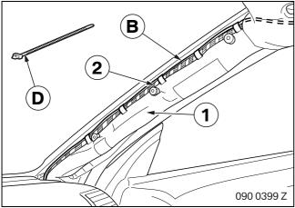
So as not to adversely affect the function of the airbag (1), secure earth cable **B** to the standard wiring harness (2) with cable ties **D**.
