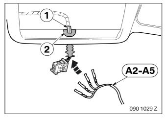
Remove the adhesive tape (1) from the rubber grommet (2).
