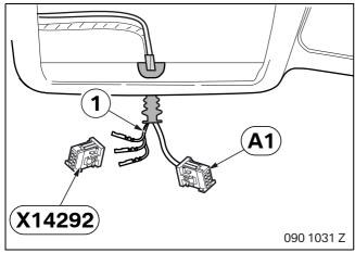
Disconnect the following cables (1) from plug **X14292** and connect them to branch **A1**:
