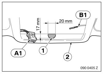
Cut out the marked area (1) of the headlining (2) using the dimensions shown.
