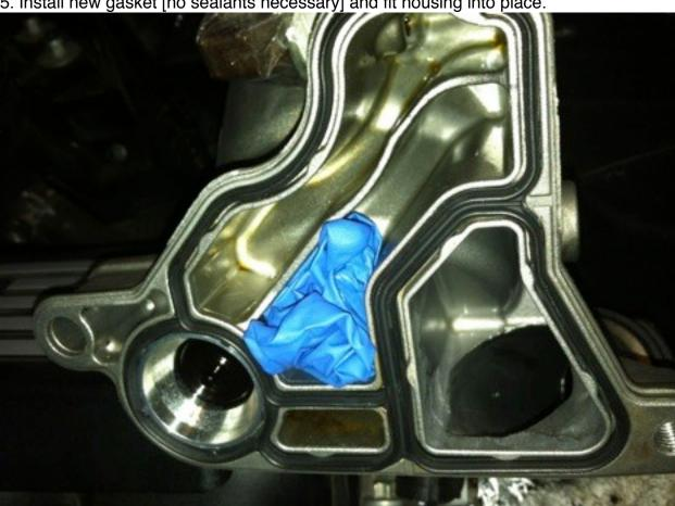
5. Install new gasket [no sealants necessary] and fit housing into place.
