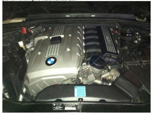
2.Remove oil filter cap, oil filter, oil, and clean with a rag. [I used a turkey baster to get the oil out and then finally wiped the excess oil with a rag]
