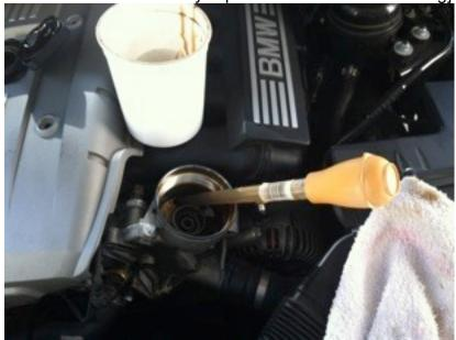
3. Remove (3) 8mm screws mounting Oil Filter Housing with 8mm box end wrench
