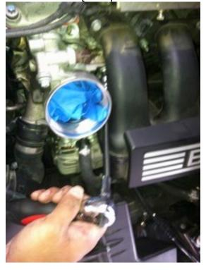
2d. With an 8mm wrench, unbolt the easiest bolt. [Notice the aluminum, I covered the alternator so that oil or coolant doesn't ruin it. I also wrapped the brown oil pressure switch with tape just in case.
