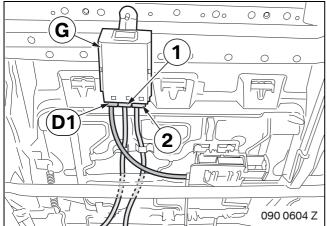
If the SW 13-pin plug (1) is not in seat disconnection plug **X279** (19-pin GE), connect branches **D2 - D5** to plug **K**. ◀
