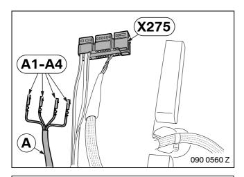
Connect driver's seat wiring harness **A** to seat disconnection plug **X275** (19-pin GE) as follows:
