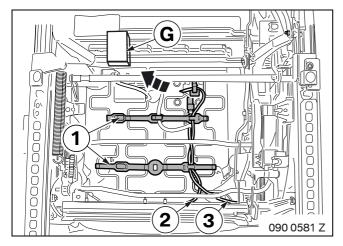
Connect the plug for the backrest heating element (1) and seat heating element (2) to seat module **G**.
