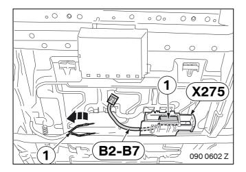
Disconnect, insulate and tie back the following cables from seta disconnection plug **X275** (19-pin GE):
