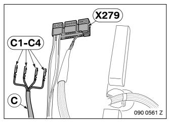
Connect passenger seat wiring harness **C** to seat disconnection plug **X279** (19-pin GE) as follows:
