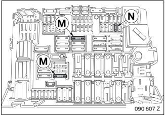
Insert 30 A fusible inserts **M** into slot F32 and F49. Insert 5 A fusible insert **N** into slot F29. Install the glove box with casing.
