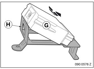
Insert seat module G into holder H and secure it.
