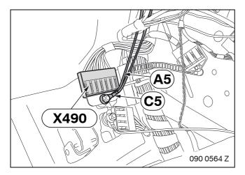
Secure branch **A5**, BR cable, and branch **C5**, BR cable, to joint connector **X490**.
