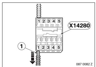
Release distributor station preparation X14280 and car distributor station X14255 behind the left backrest part.
