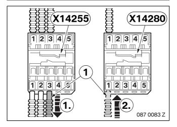
Disconnect any bottom FO conductor (1) from car distributor station **X14255** and connect it to PIN 1 of distributor station preparation **X14280**.
