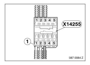
Connect the FO conductor (1) that you disconnected from distributor station preparation **X14280** to the cleared PIN in car distributor station **X14255**.
