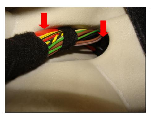
5. The harness routes through the passenger rear seat area into the trunk, as shown in the picture. Ensure that the harness is properly routed through the grommet.
