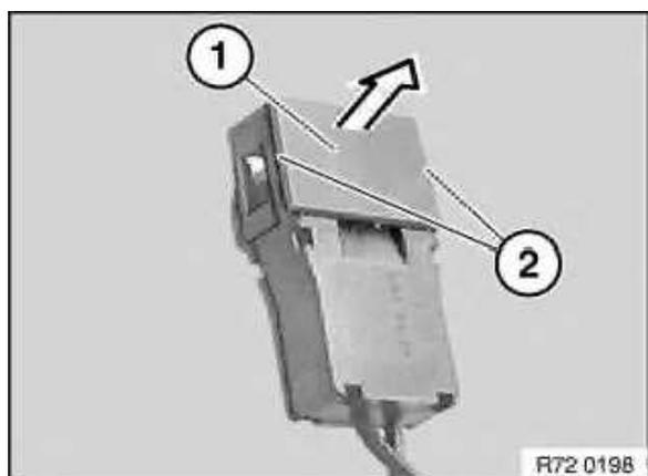
**Airbag plug connection on gas generator/airbag module offset by 90°:**
