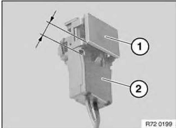
Cover (1) is not positioned higher than housing (2). The airbag plug connection is unlocked and can now be detached from the gas generator/airbag module.
