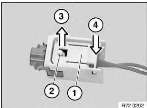
**Airbag plug connection on gas generator/airbag module is straight (2 versions)**
