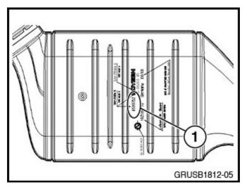
Check the part number of the SCR catalyst (1). If the part number is not 18 30 8 509 752/753 (E70) or 18 30 8 509 749/750 (E90), the SCR catalyst will need to be replaced.
