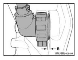
an indication of an incorrectly installed sealing sleeve!!!
