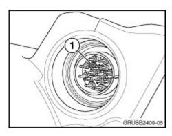
5. In some cases, the incorrectly installed sealing sleeve may permanently damage pins in the Mechatronic connector (X8500). In such a case, the Mechatronic module has to be replaced (**pin repair is not possible**).
