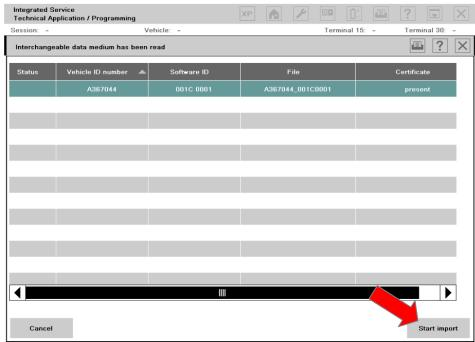
The VIN and Software ID should be visible in the next step. Select the codes you want to import and use the Start import button.
