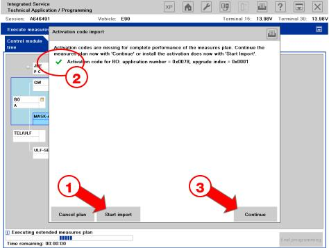
11. The second option to import Enabling Codes into ISTA/P is during a programming session. If codes are needed, and have not been imported previously in data management, ISTA/P will prompt for the Activation code import. Insert the USB stick or the CD-R, and select the Start import button. When the code is imported correctly, you'll see a green mark. Select continue to proceed with programming.
