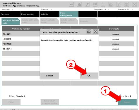
8. There are two options to upload Enabling Codes to ISTA/P. The first option is in the Data managemet-tab/ Import activation code tab. Select the Import button. ISTA/P will ask you to put in the USB-stick or CD-R. Confirm with "OK".
