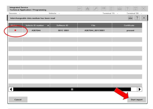
10. In the next screen, the codes will be marked with a red dot. Select the codes to be imported again and use the Start import button again. In this step, the certificates are imported into ISTA/P.
