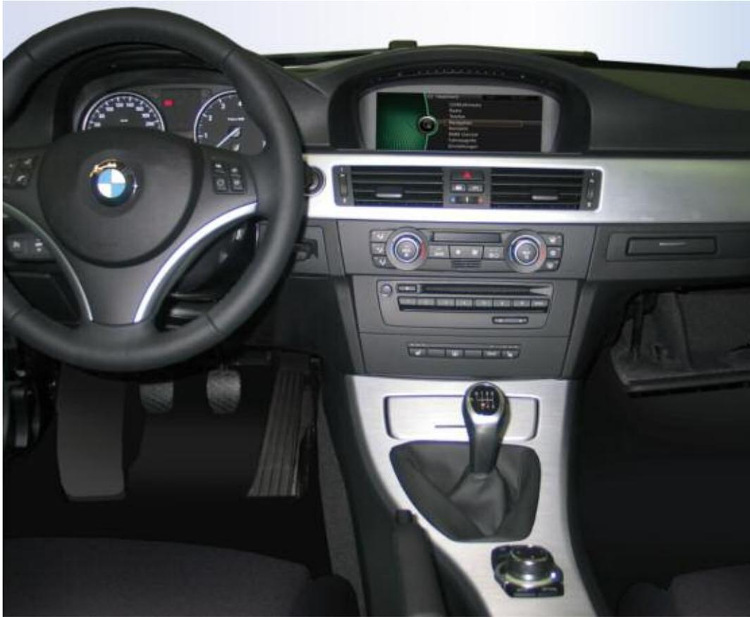
**iDrive system with CIC on an E90 vehicle**
