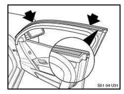
Movement between the flocking material (felt-like material indicated by the arrows) on the upper door seal and the surrounding roof panel may produce squeaking or creaking noises.
