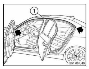
Apply a continuous length of Teflon tape
