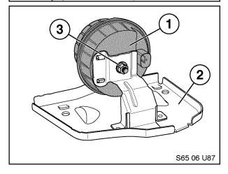
6. Position siren (2) to mounting plate (3) and secure in place with M6 hex nut (1).
