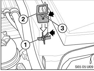
3. Position hood switch bracket (2) to mounting location (1) and secure in place with ST 4.8x 13 screw (3).
