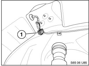
3. Locate 6-position black siren connector (1) in upper LH wheel arch area. Remove securing tape.
