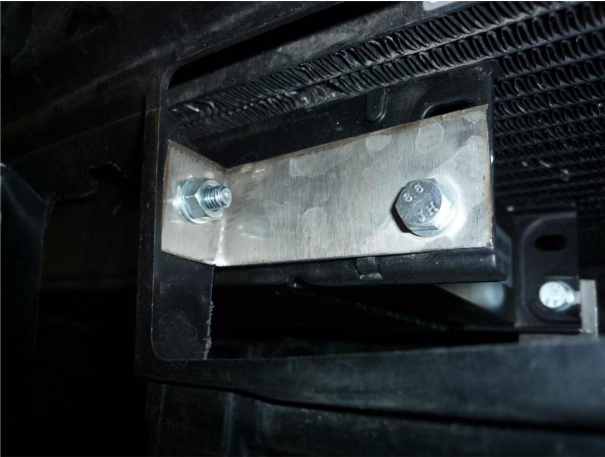
Now cut a hole for the two oil lines in the lower portion of the shroud. The hole we cut is much larger than needed, and was partially already there from some other R&D. You can cut it quite a bit smaller. Oil lines are routed in between the radiator and the chassis. There is a nice gap that allows lines to pass.
