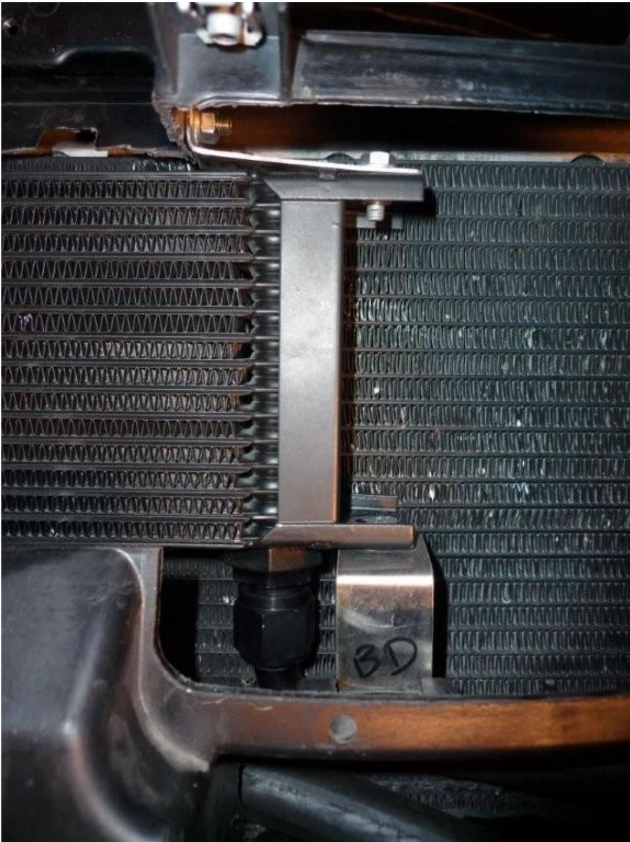
View from top looking down on right side, hole is drilled to side of center brace that was trimmed.
