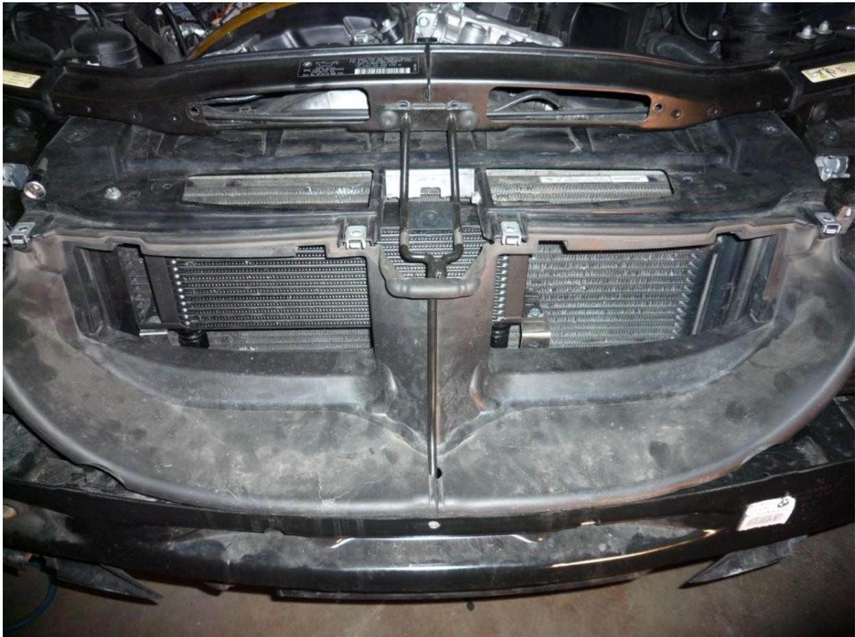
5. Now you will need to trim out the center plastic brace. Assemble brackets to oil cooler, drill mounting holes using the oil cooler with brackets as a template. When you are done, it will look like this:
