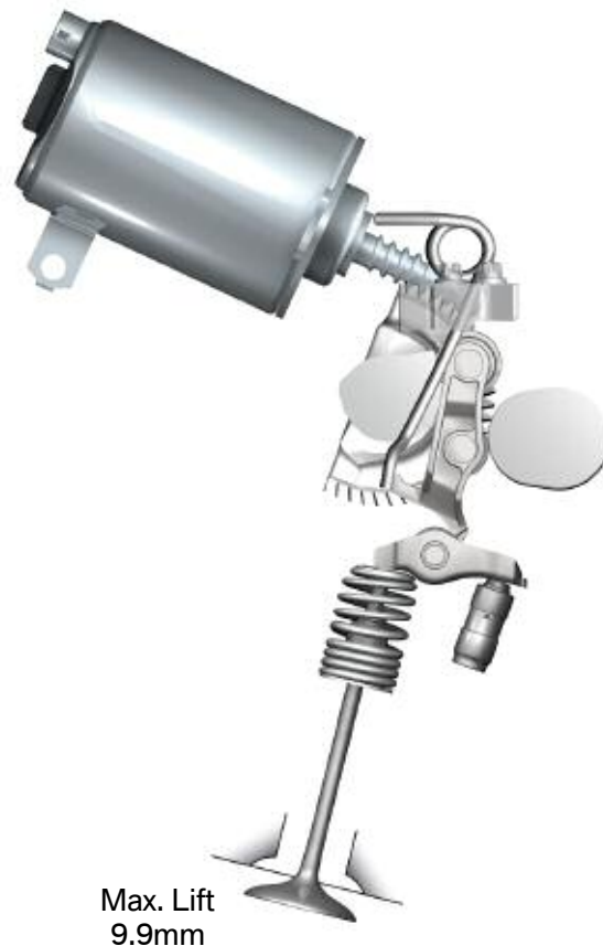
Valvetronic II at maximum valve lift
