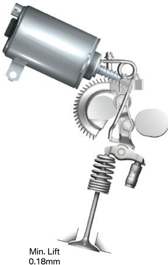
Valvetronic II at minimum valve lift
