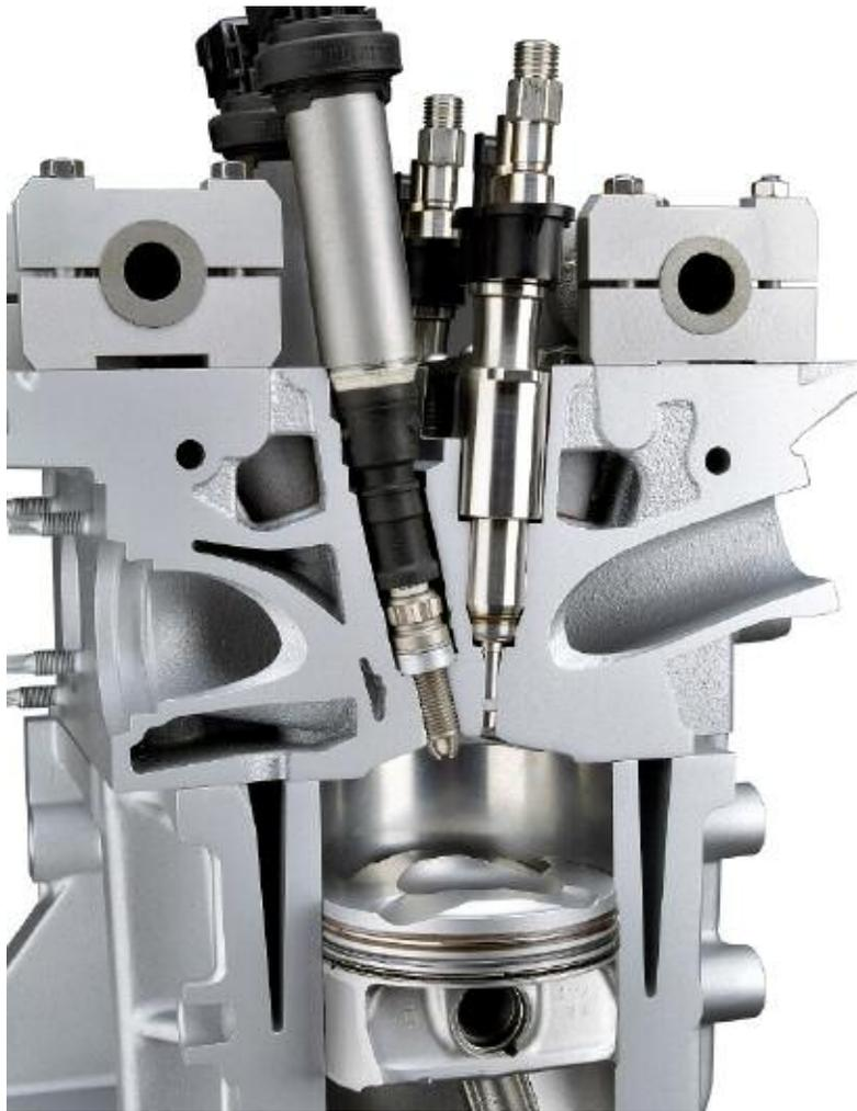
High precision injection allows for a more precise metering of the fuel injection process and therefore permits a higher compression ratio of 10.2 to 1. This compression ratio is quite high considering the N54 is turbocharged. However, the "spray guided" injection process cools the air charge and decreases the possibility of unwanted engine knock. The operating pressure of the HPI system is up to 200 bar.
