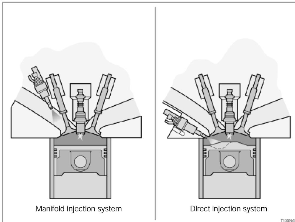
The DI system allows for increased engine efficiency and has several distinct advantages over manifold injection systems:
