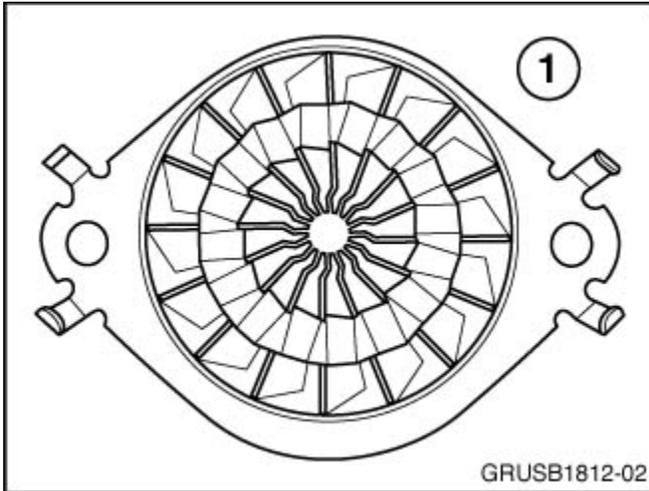
The original style mixer has a multiple fin arrangement (1). This mixer will need to be replaced with P/N 18 30 8 513 445 (E70) or P/N 18 30 8 512 438 (E90).
