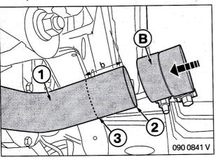
Mark the entrance pipe (1) from the cut end (2) with a distance of  $\mathbf{b} = 35 \text{ mm}$  (3).
