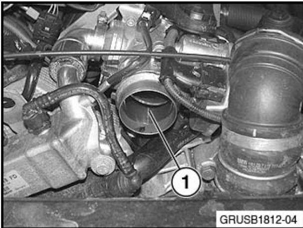
Remove the charge air pipe at the throttle (ignition off). Using a flashlight, look through the throttle (1) and inspect the EGR valve.
