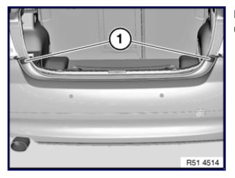
Lever out cover (1) and release screw underneath.
