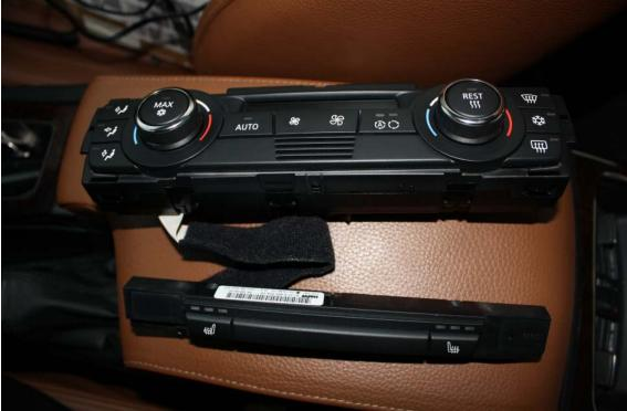
6. Now that both are separated you can focus on getting the CD player out. Remove the two Phillips head screws at the bottom side to release the unit.
