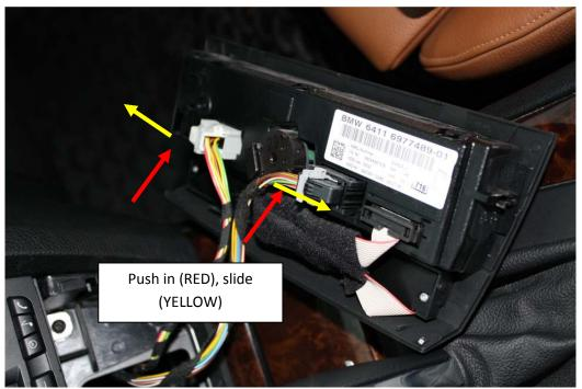
4. Now you need to remove the climate control module from the trim piece. Do this by releasing the clips as illustrated. The clips are the same on the top and bottom.
