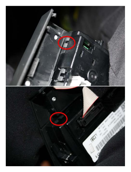
5. Now you should have separated the climate control module from the trim piece like the picture below. Now remove the seat heater controls by releasing the tabs indicated.
