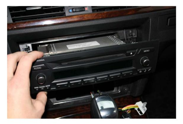
7. Now remove the cables to the back of the stock headunit. They are one main harness and one antenna adapter. For the main harness you need to just pry up on it slightly with a flathead and then it will rotate back and push the connector out. For the antenna adapter just push in on the passenger side and pull out.
