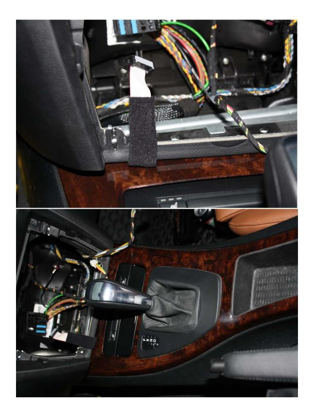
22.In order for the stock climate controls to fit into the Dynavin housing they need to be trimmed as shown in the pictures.
