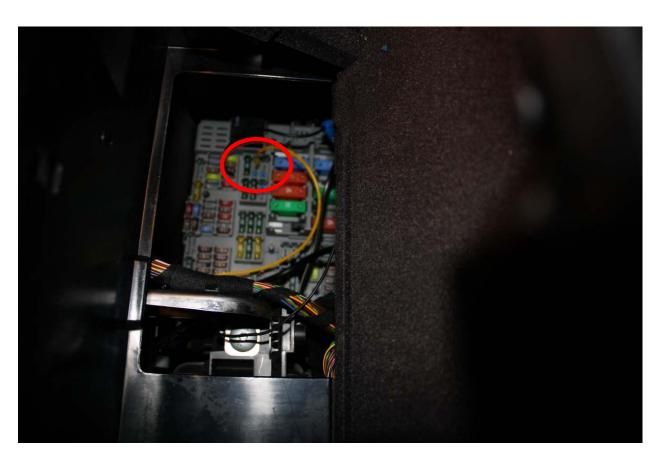
26. Now connect the harnesses to the CANBUS box as pictured below. Connect the antenna adapter as well. Mount the GPS Antenna as pictured on the metal tube, it will get signal here!
