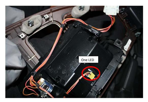
16.To get out the cigarette lighter is a tricky process. If you look closely you can see tabs that hold it into the ashtray housing. You need to get small flathead screwdriver and press these in while applying pressure to push it out the top of the ashtray. With some persuasion you can get it done but it does take some time.
