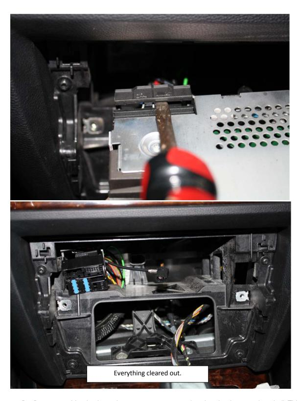
8. Once everything is cleared out, move onto removing the plastic mounting shell. This is held in by 4 Torx T15 screws and two bolts on the bottom. Shown below;
