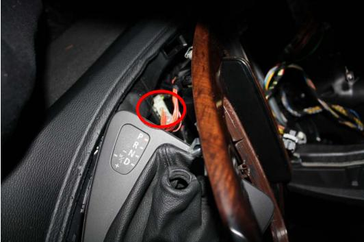
13. Now disconnect the clips to the ashtray as pictured above and below. Press the sides in and slide away to remove the clip.
